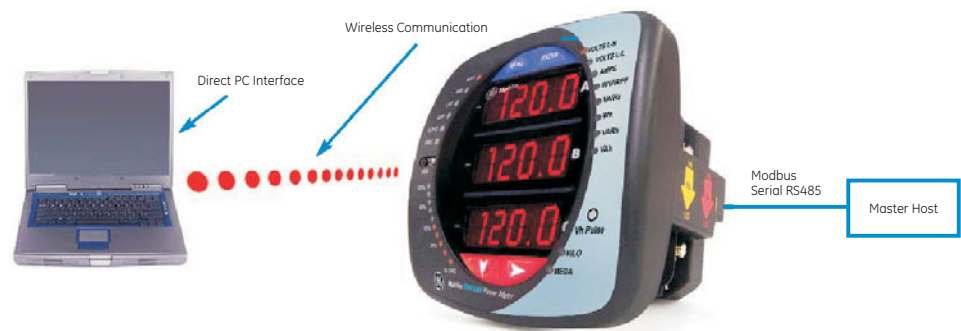
FIGURE 3–15: Simultaneous Dual Communications Paths
